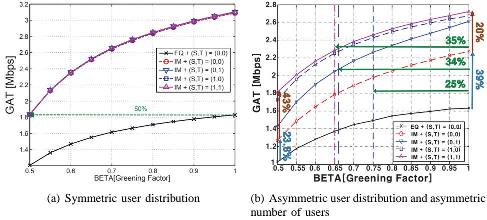
Fig. 6. GAT of four Greening frameworks and equal power allocation with no power sharing
