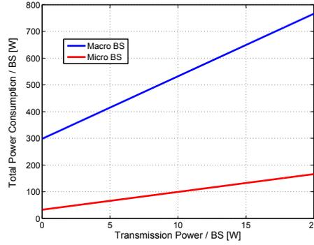
Fig. 1. Total power consumption vs. transmit power
