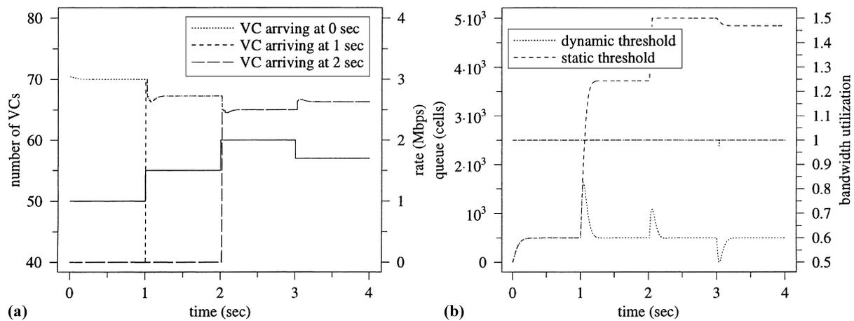
Fig. 6. Control performance upon arrivals and departures of VCs ( $\mu = 150$  Mbps,  $\tau_i \in [10, 40]$  ms,  $B = 5000$  cells,  $K_i = 10.0 \forall i$ ): (a) trajectories of number of VCs (solid curve) and  $r_i(t)$  of VCs arriving at 0, 1, 2 s in the case of FRFC with DQT; (b) trajectories of  $q(t)$  and bandwidth utilization.
