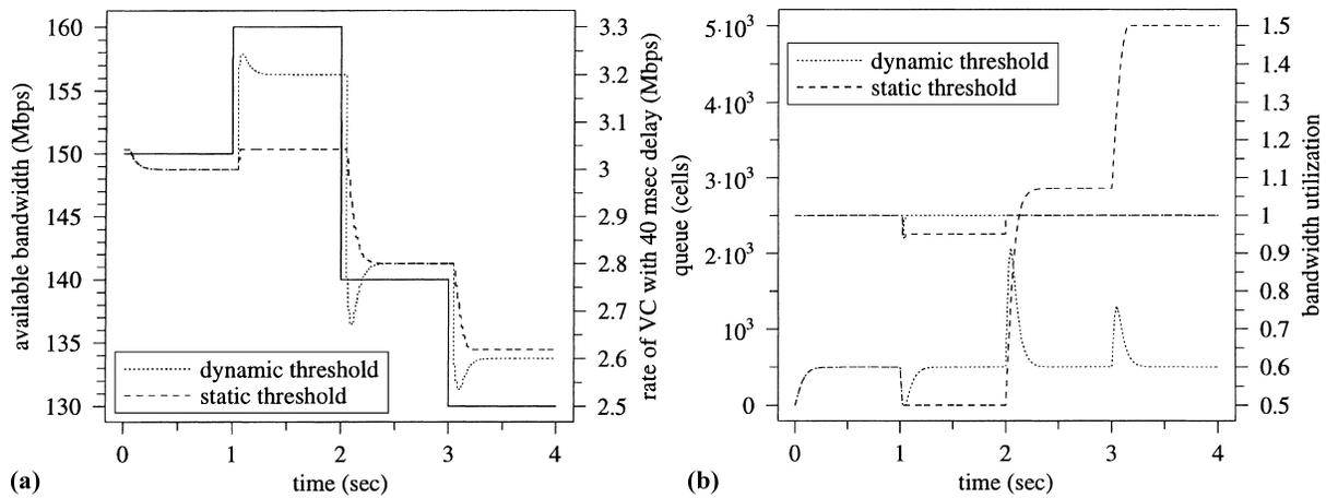
Fig. 5. Control performance when  $\mu(t)$  is piecewise constant (no. of VCs = 50,  $\tau_i \in [10, 40]$  ms,  $B = 5000$  cells,  $K_i = 10.0 \forall i$ ): (a) trajectories of  $\mu(t)$  (solid curve) and  $r_i(t)$  of a VC with 40 ms round-trip delay; (b) trajectories of  $q(t)$  and bandwidth utilization.
