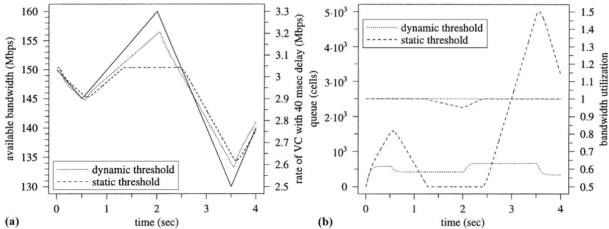
Fig. 4. Control performance when  $\mu(t)$  is continuously varying (no. of VCs = 50,  $\tau_i \in [10, 40]$  ms,  $B = 5000$  cells,  $K_i = 10.0 \forall i$ ): (a) trajectories of  $\mu(t)$  (solid curve) and  $r_i(t)$  of a VC with 40 ms round-trip delay; (b) trajectories of  $q(t)$  and bandwidth utilization.
