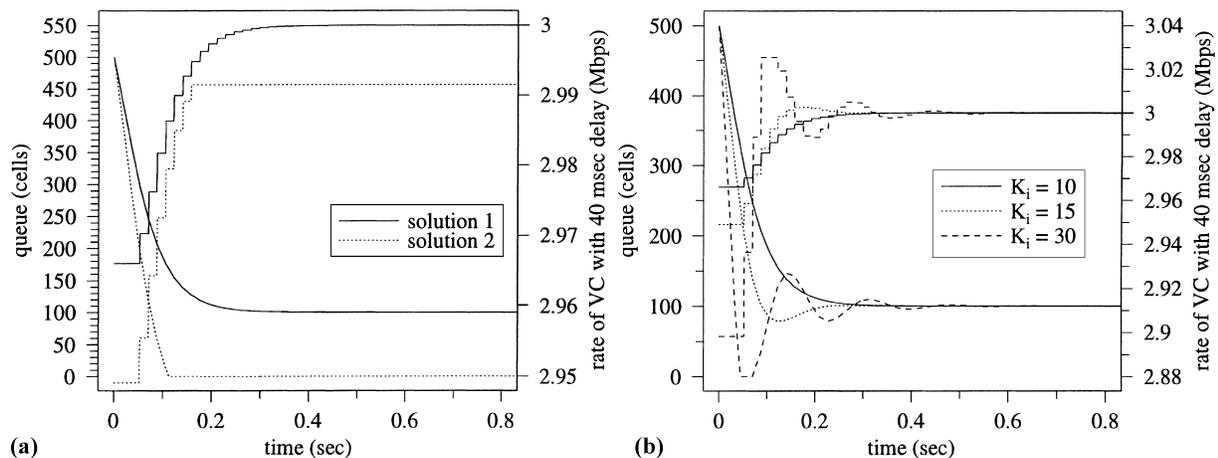
Fig. 3. Control performance in static environment ( $\mu=150$  Mbps, no. of VCs=50,  $\tau_i \in [10, 40]$  ms,  $B = 5000$  cells): (a) two steady-state solutions with  $K_i = 10.0 \forall i$ ; (b) effect of control gains  $K_i$ .
