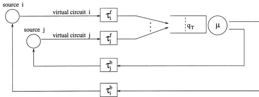
Fig. 1. Network model with a single bottleneck link.
