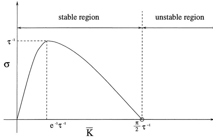
Fig. 2. Dependence of asymptotic decay rate  $\sigma$  on control gain  $\bar{K}$  for given round-trip delay  $\tau$ .
