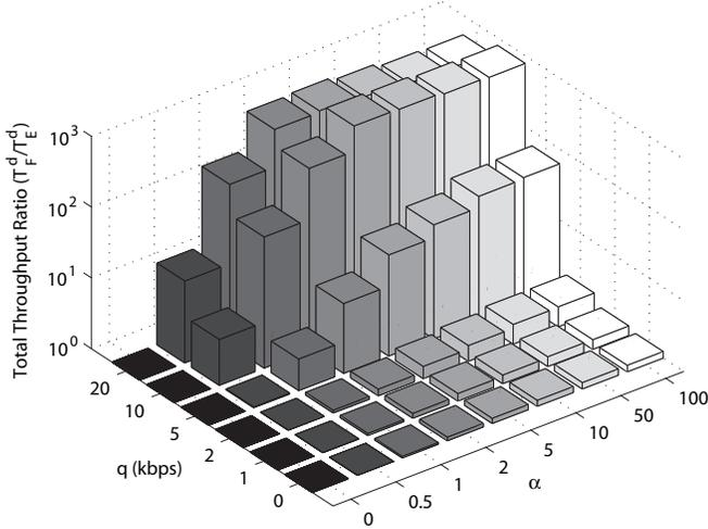
Fig. 7. Impact of discrete rates on EPA ( $T_F^d/T_E^d$ ): FPA vs. EPA ( $s = 6$  and  $B = 20\text{MHz}$ ).
