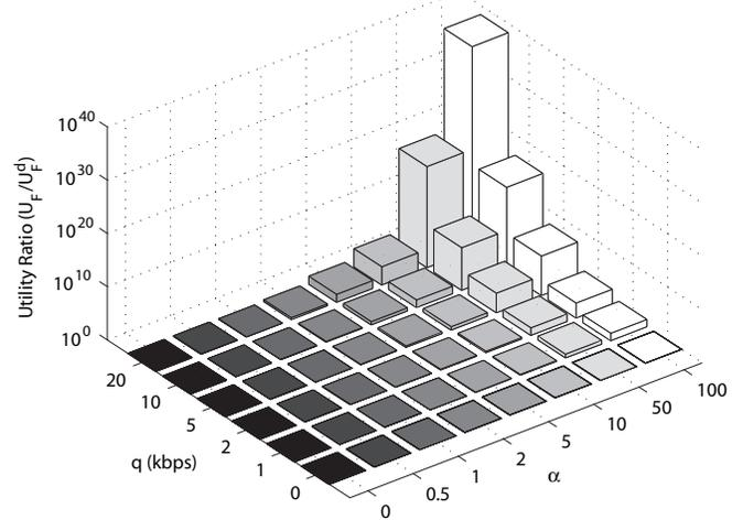
Fig. 6. Performance degradation of FPA ( $U_F/U_F^d$ ): continuous vs. discrete ( $s = 6$  and  $B = 20\text{MHz}$ ).
