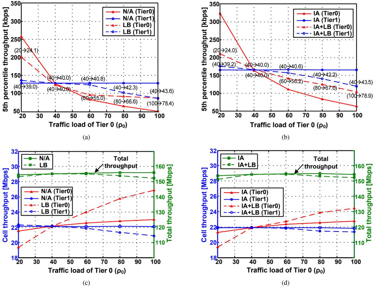
Fig. 5. System performances with different four schemes (N/A, LB, IA, IA+LB): (a),(b) 5th percentile throughput and (c),(d) cell and total throughput.
