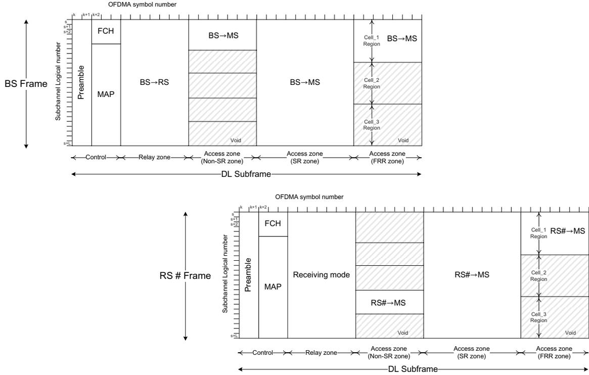
Fig. 2. Proposed frame structure for MCN
