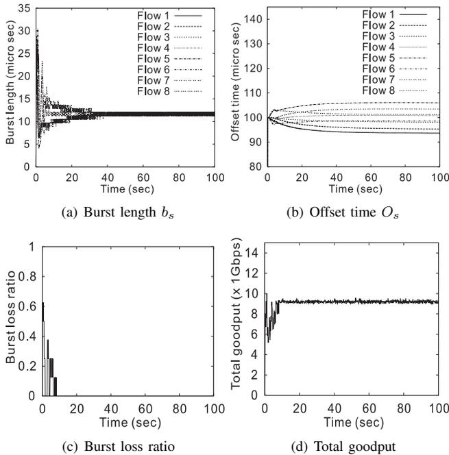
Fig. 4. Simulation results in single link scenario: convergence to the state of zero loss and maximum goodput.
