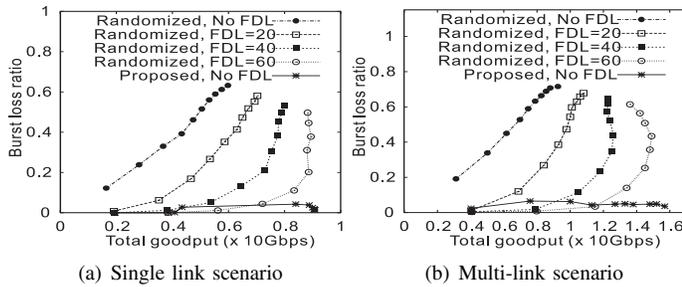
Fig. 6. Comparison of the proposed method and conventional methods while increasing offered load: In conventional methods, the goodput performance is increased only at the cost of high burst ratio. Proposed method is keeping very low burst loss ratio even at the highest goodput.
