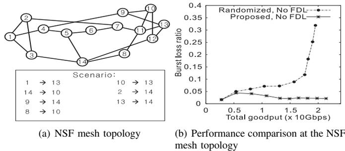
Fig. 7. Comparison of the proposed method and the conventional method at the NSF mesh topology. The proposed method outperforms in terms of burst loss ratio and goodput.
