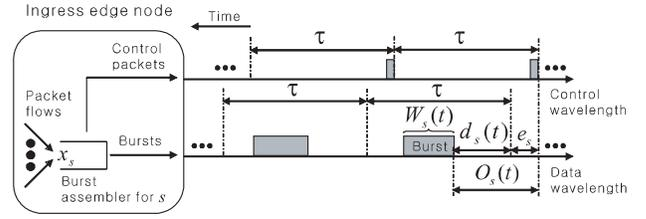
Fig. 1. The time diagram for departure of both control packets and bursts of the flow  $s \in S$  in ingress edge node: The burst with its duration  $W_s(t)$  (sec) and its control packets are sent every burst assembly time  $\tau$  (sec).
