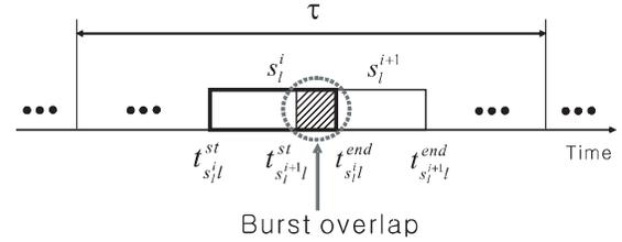
Fig. 2. An example of burst overlap: In a single wavelength in link  $l$ , burst overlap occurs when the end time of a burst is later than the start time of its consecutive burst. The burst flow sources denoted by  $s_l^i$  and  $s_l^{i+1}$  are named by the order of arrival times of their control packets.
