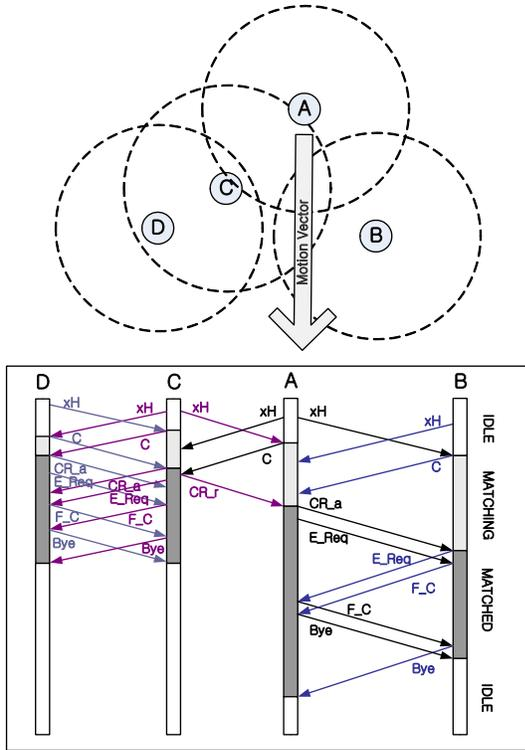
Fig. 1. Protocol procedure : when all the nodes try to match
