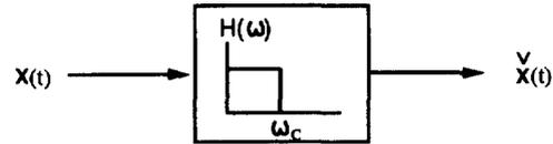
Figure 2: A low-pass filter
