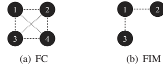
Fig. 2. Example topologies' conflicting graphs. Vertices are the links in interference graphs; dotted lines represent interference; (a) FC with 4 links; (b) FIM with 2 outer links.
